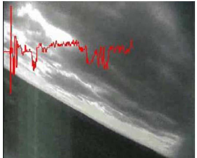
Fig. 8. Angle of roll measured during flight
