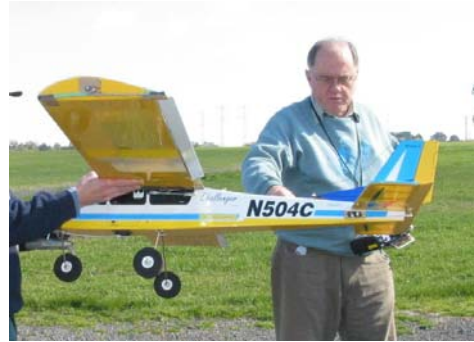
Figure 12. Controls ground test. Note the aileron & elevator deflection while the vehicle is stationary.
