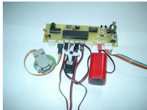
Figure 14. Digital section with ASI and Altitude sensors, servo, RS-232 interface and battery pack.
