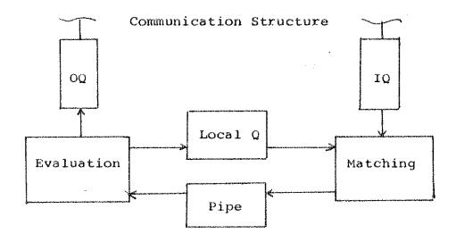
Figure 3.1 Processing-element
