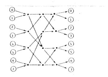
Figure 3.3 Rectangular Shuffle Network (8 elements)
