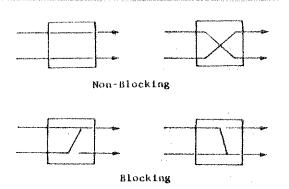
Figure 3.2 Router Block Configurations
